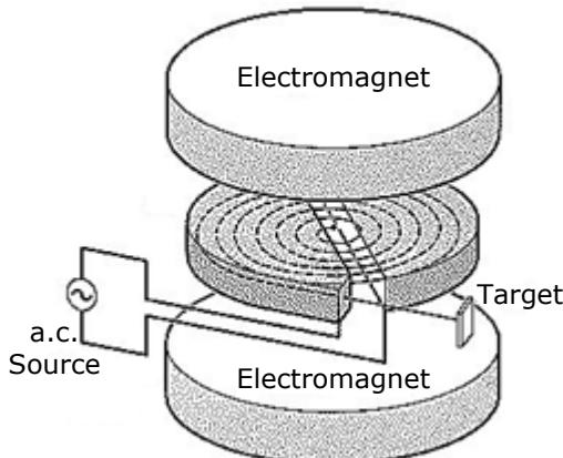
Cyclotrons are located in the same hospital as the PET scanners and are used to manufacture radioactive nuclei. Cyclotrons are circular devices in which charged particles are accelerated in a spiral path within a vacuum. The particles are accelerated by a rapidly alternating voltage and acquire high kinetic energies. They spiral outwards under the influence of the magnetic field until they have sufficient velocity and are deflected into a target producing radioactive nuclei, including carbon-11.
